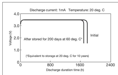
\* Nominal capacity indicates duration until the voltage drops down to 3.0V when discharged at a nominal discharge current at 20 deg. C.
